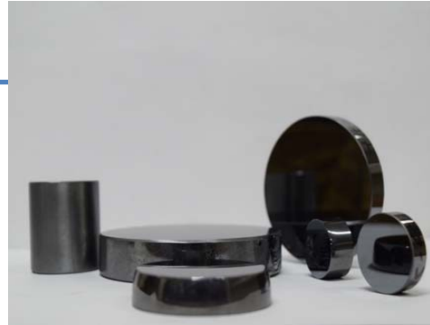
Processed bigger \text{As}_2\text{Se}_3 glass (varied dimensions)
